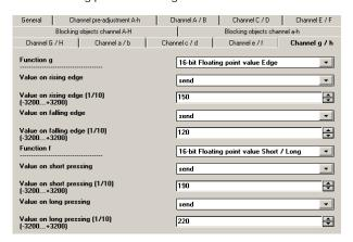
The function is used to send 16-bit floating point values (FP values as EIS 5) ranging from -320.0...+320.0, with one decimal place. In the process, the exponent of the 16-bit FP value is fixed at the value "4". An adjustment can be made as to whether a value telegram is to be sent as a reaction to a rising and / or falling signal edge on the channel input (i.e. when a push button is pressed and / or released).
