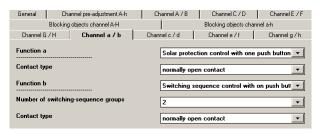
The channel can be used for 1-button solar protection control. A distinction is made between short and long push button action.
