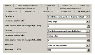
For binary inputs, this function enables the counting and saving of pulses as 8-bit counter value. The counter value stored in the counter value object can be sent on request and after modification by a configurable differential value. Where required, the counter value can be reset to value 0 by telegram via an additional 1-bit communication object. Adjustments can be made via parameters as to whether the counter status should be incre-
