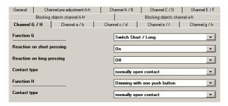
This function is used, for binary inputs to which a switch or a push button is attached, to send a switching telegram (ON, OFF or TOGGLE) as a reaction to a short or long push button action.
