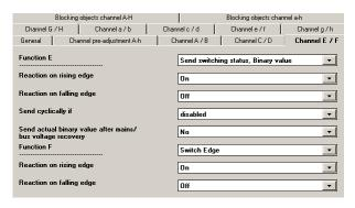
This function is used, for example, to query and transmit the switching status of a signalling contact or the voltage level present at a channel input. Adjustment via this parameter defines which binary value is to be sent after a status change, whether the switching status / binary value is to be sent cyclically in addition and whether the current switching status / binary value is to be sent automatically even after bus or mains voltage recovery.
